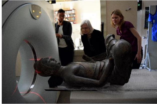
Computed tomography scanning of the Freer Gallery of Art's lacquer buddha at the National Museum of Natural History. Image by Freer | Sackler staff
