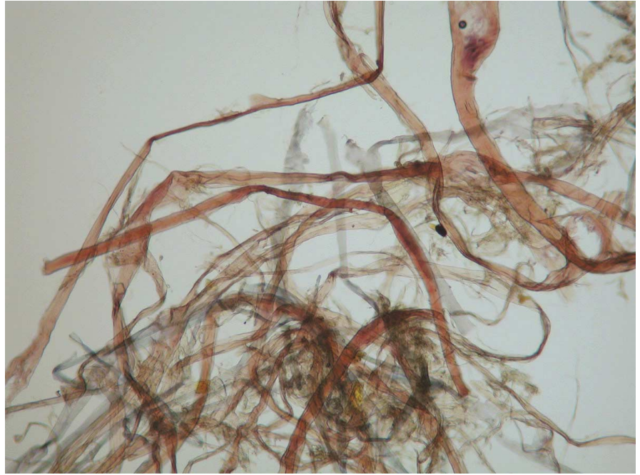
Fig. 2 Fibre sample taken from May 1 st Sutra (F2002.9f) stained with Graff's C-Stain. Ramie fibres seen in red and gampi fibres seen in greenish-blue. Photomicrograph.
