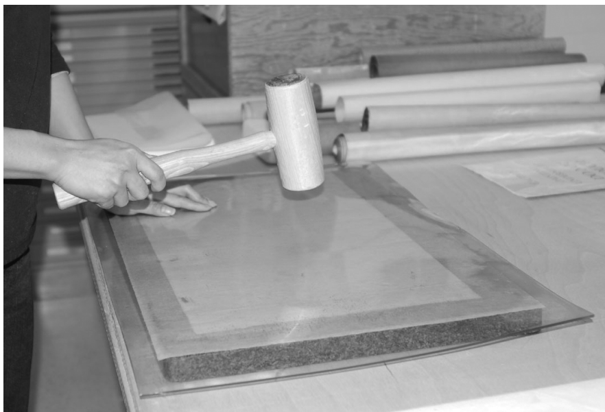
Fig. 4 A stack of dyed and thinned sheets of repair paper being hammered to produce crisp, dense paper, with a smooth surface, characteristic of uchigami .
